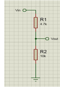
Figure 4: Voltage divider for sampling
